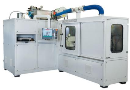
Autofrettage machine for prototypes
