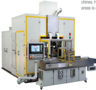
Autofrettage machine for serial production
